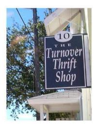
(c) *Under canopy sign.* A sign hung from a canopy or roof of a walkway. It may be rigid or it may swing. Such a sign may not have more than two sign faces.
